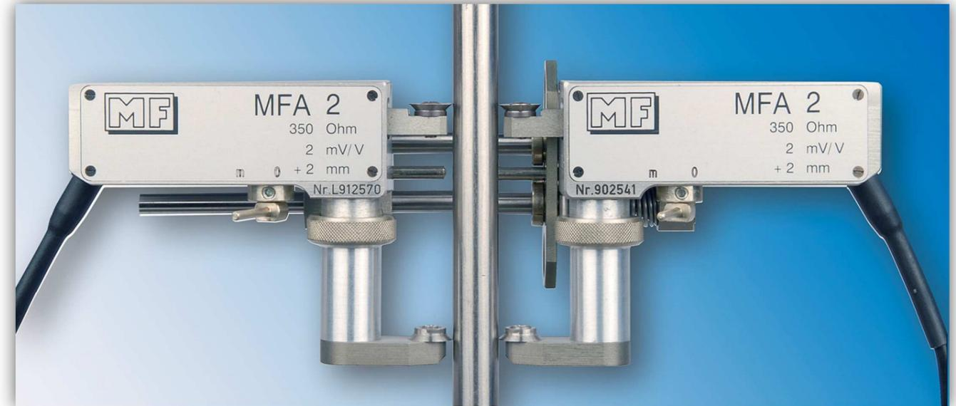
Picture 2: MFA 2 – double-sided extensometer
